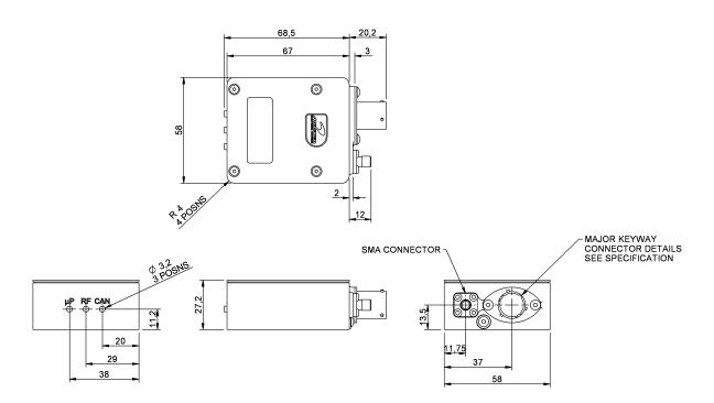
Description Order Code Drive plate receiver O 030 205 005 000 Receiver ANA/CAN/PWR connection cable O 030 205 990 000 O 030 205 990 004 1.5m antenna extension cable
